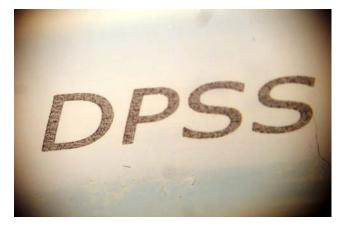
Many applications call for specialty plastic tubing to resist chemicals, acids, hot solvents and heat. Often it is difficult to print directly on these materials and labels are an ineffective solution. Many of these plastics can be marked directly with a 355 nm DPSS Laser. 355 nm lasers offer several advantages over typical IR and CO<sub>2</sub> lasers for marking these devices.
