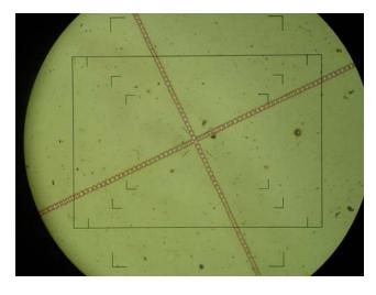
Indium-Tin Oxide (ITO) removal and patterning on glass and plastic is a rapidly growing application for DPSS 355 nm lasers.
