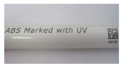
ABS Marked with DPSS Lasers Inc. 355 nm UV Laser ABS, acrylonitrile butadiene styrene is a light, rigid thermoplastic. It is often used to manufacture piping, musical instruments, automotive body parts, medical cases, protective headgear and golf club heads. It is most often chosen because of its high impact resistance, hardness, high gloss, slippery surface and electrical insulation properties.
