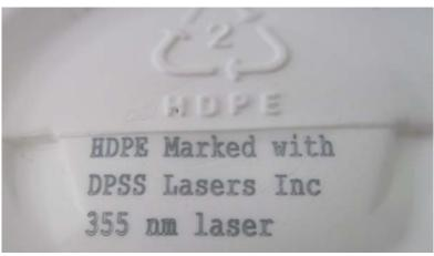
DPSS 355 nm UV lasers are able to affect a mark on many types of HDPE via a photochemical process. This "Cold Marking" process eliminates the thermal damage typically encountered with longer wavelength lasers. The resulting mark becomes a permanent part of the product and requires no inks or solvents. Because many plastics are extremely sensitive to UV wavelengths, marking speeds of 3 to 5 meters per second are achievable with UV powers as low as a few hundred mW.
