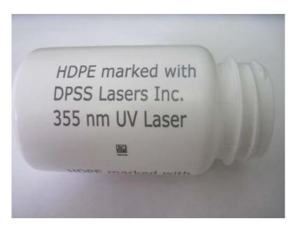
HDPE, high-density polyethylene is often selected for its strong intermolecular forces and high tensile strength. It is used in products and packaging such as medical and pharmaceutical containers, milk jugs, detergent bottles, garbage containers, food storage and water pipes.
