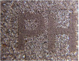
Laser marking on metals has long been a domain of IR and CO<sub>2</sub> lasers. The marks are the results of thermal modification of the metallic structure.
